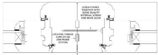
SEAL FRONT FACE WITH GOOD QUALITY EXTERNAL GRADE SEALANT
